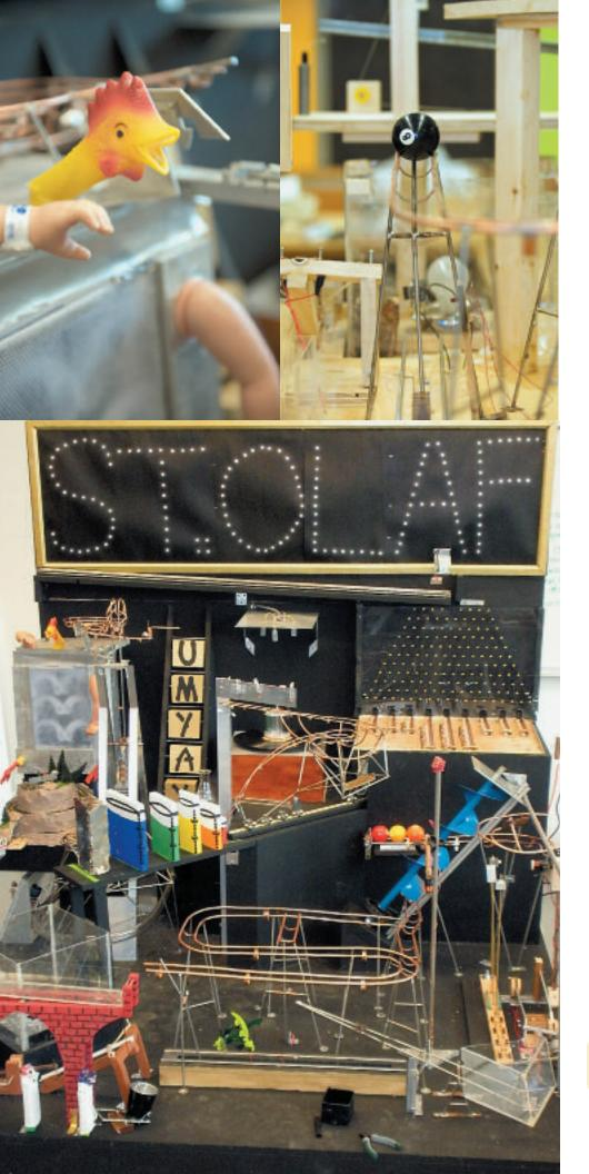
The St. Olaf team built a spinning turntable that rotates an LP record with three holes. When lined up perfectly, these holes emit lasers beams that open three gates to allow a ball bearing to roll down a copper track, eventually triggering a sign with the letters "U-M-Y-A-Y-A." As the machine's sequence ends, metal balls filter through a Plinko board triggering tiny LED lights that spell "St. Olaf."
