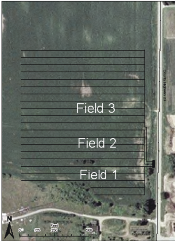
Figure 1 – Map of study site showing tile drainage. The three output pipes drain the three fields (Field 1 at the south, Field 2 in the middle, Field 3 at the north) treated with different fertilizer type and quantity (St. Olaf College Agricultural Lands, October-November 2009).
