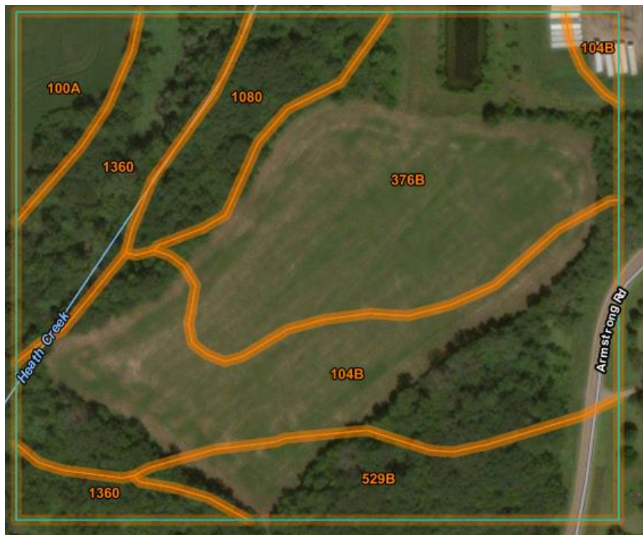
Fig. 11. Soil map for Heath Creek site. 376B corresponds to Moland Silt loam soil type, 104B is Hayden loam, and 529 B corresponds to Ripon silt loam.
