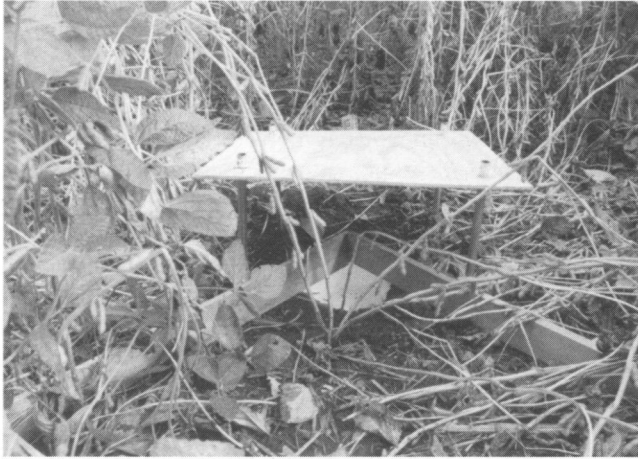
Figure 1. A catch-basin constructed to assess the effects of agriculture (rotation soybean field) on soil runoff. Catch-basins consisted of a bucket, 9 in. (23 cm) in diameter, placed into a hole dug in the ground, beneath a raised plywood shelter. The shelter ensured that no rainwater would enter the bucket directly, and therefore that all water collected represented surface runoff from the fields. Pieces of plywood, 4 ft (1.2 m) long, were placed to form a 90° angle with the bucket at its vertex. This standardized the width of the collecting area to approximately 5.7 ft (1.7 m).
