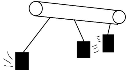
To set up the experimental equipment, measure out three strings with lengths 10 cm, 20 cm, and 30 cm. Attach a mass to one end of each string and attach the other end to the rod so that all three masses are hanging from the rod like pendulums of different lengths, like the figure above.
